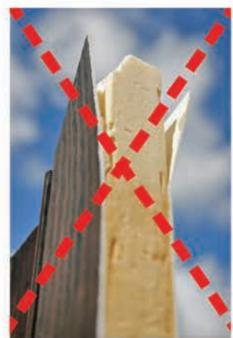
The Picture above shows conventional composite doors, comprised of two 2mm skins bonded to a foam core.
