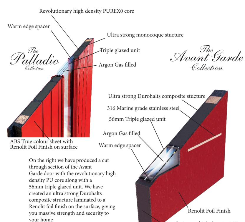
Revolutionary high density PU core
